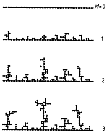
Figure 1. Clusters generated in a small scale Monte Carlo simulation. As the number of particles M added by a diffusion controlled aggregation process is increased, the relatively small clusters stop growing since they become suppressed by the neighbouring larger clusters. In this figure M denotes the number of particles in the deposit normalised by the length of the substrate.
